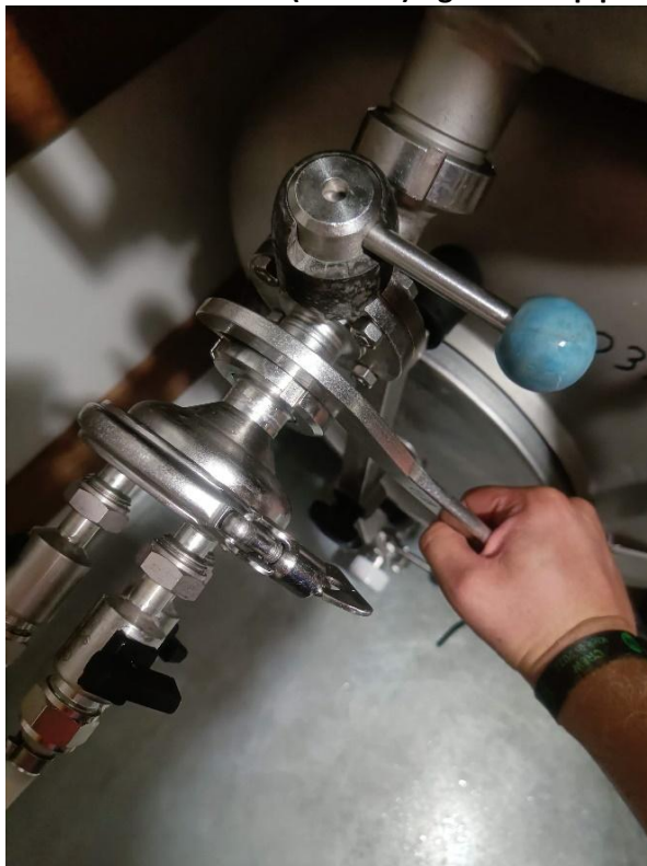
6. Use the wrench to (HAND!!) tighten the pipe 7. Pull the handle a bit and rotate it 90 degrees
