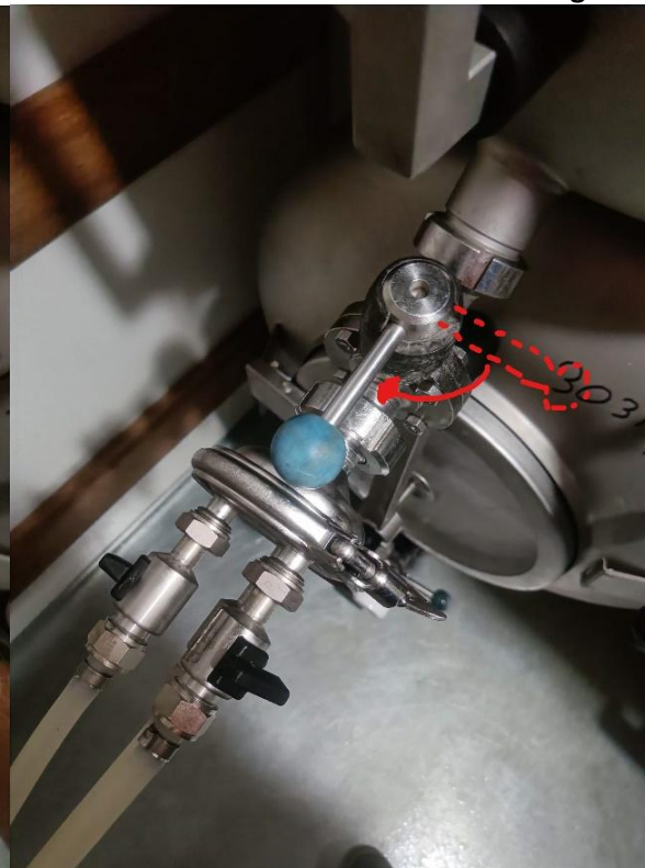
6. Use the wrench to (HAND!!) tighten the pipe 7. Pull the handle a bit and rotate it 90 degrees
